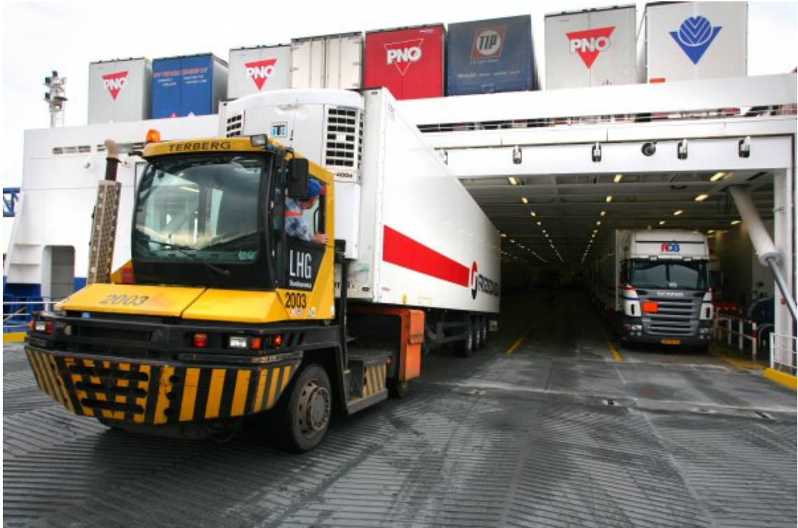
Picture 5. Trailer being loaded in to ro-ro vessel by tow master (Finnlines 2015a).
