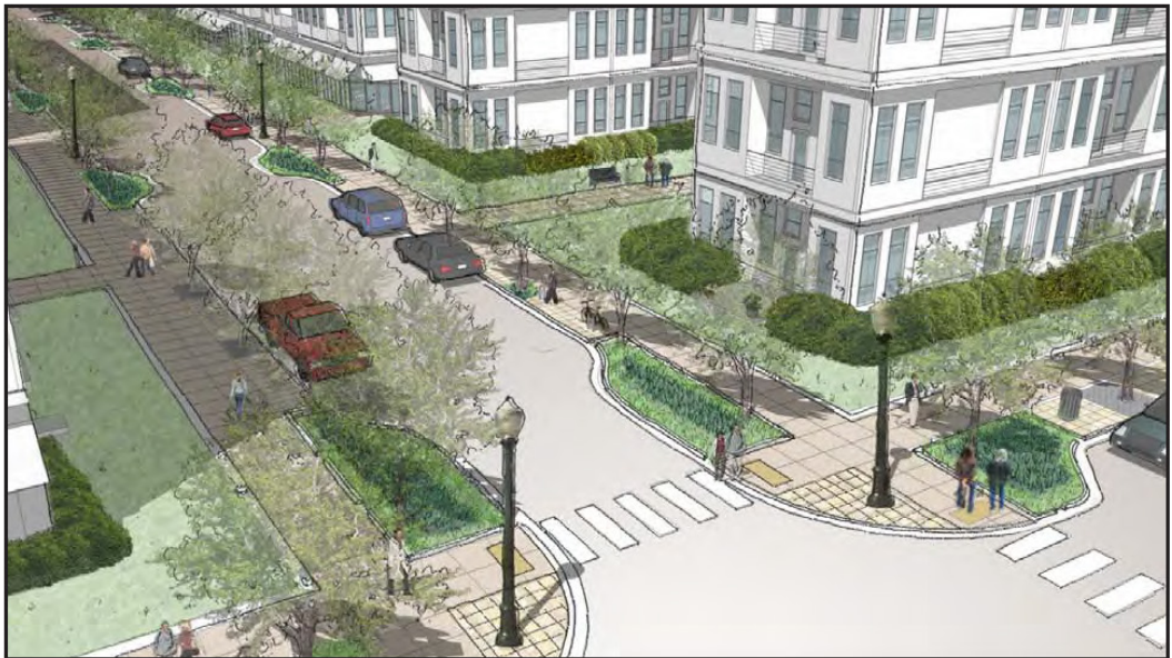
FIGURE 3: Example on green street system with storm water curb extensions. (Gateway Green Streets master plan 2008)
