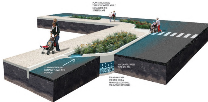
FIGURE 5: View of storm water curb extensions. (City of Philadelphia Green Streets Design Manual 2014)
