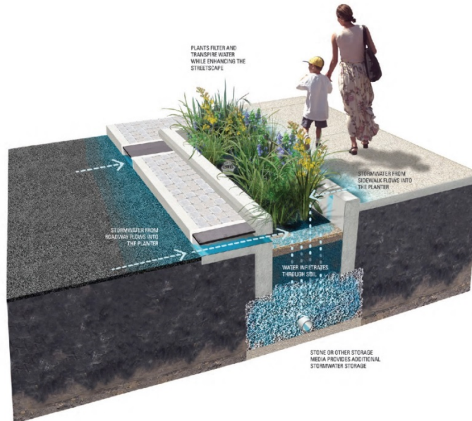
FIGURE 4: View of storm water planter. (City of Philadelphia Green Streets Design Manual 2014)
