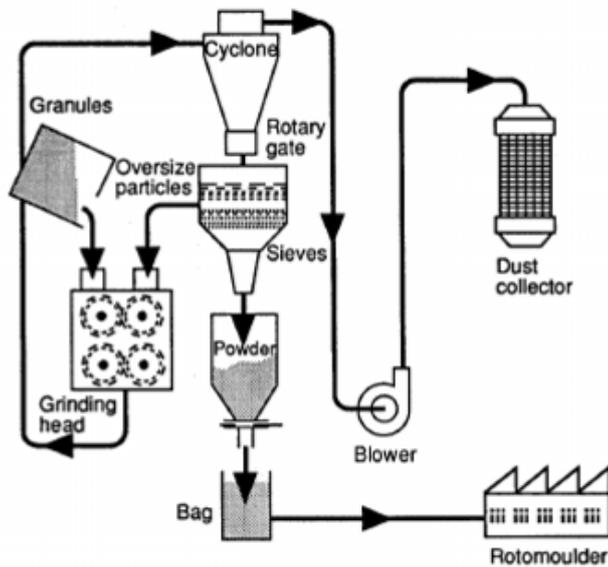
Figure 2. Stages in the grinding of powders (Crawford and Kearns, 2003)
