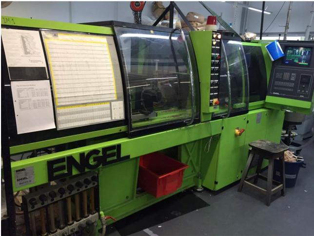
*Figure 15. Engel Injection Molding machine*
