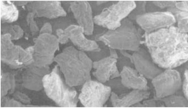
*Figure 3. Good particle shapes for rotational molding powders (Crawford and Throne, 2002)*
