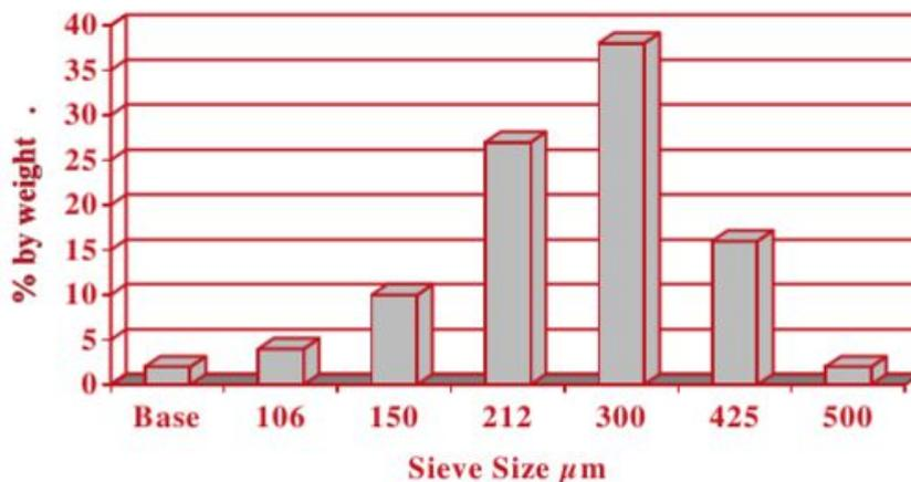
Figure 4. Typical particle size distributions for polyethylene (Crawford and Kearns, 2003)
