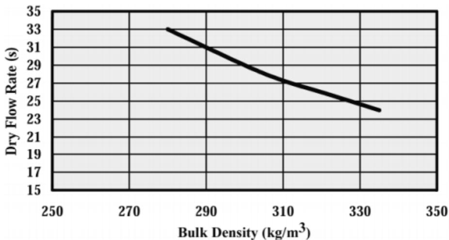
Figure 5. Variation of dry flow rate with bulk density for rotomolding powders (Crawford and Throne, 2002)
