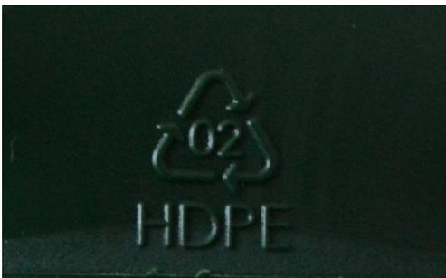
*Figure 6. HDPE identification code*
