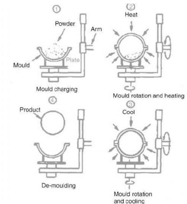
Figure 1. Principles of rotational molding of plastics (Subramanian, 2011)
