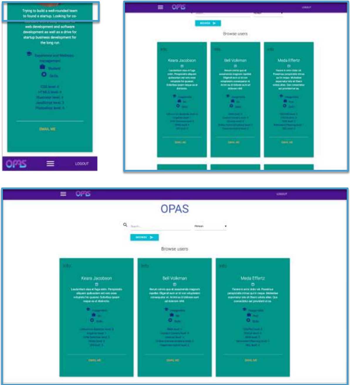
Screenshot 4. View of browse.html page in responsive layouts with breakpoints for mobile, tablet and desktop screen sizes. (Developed by the Software Engineering Project team SYS4TF222-1.)
