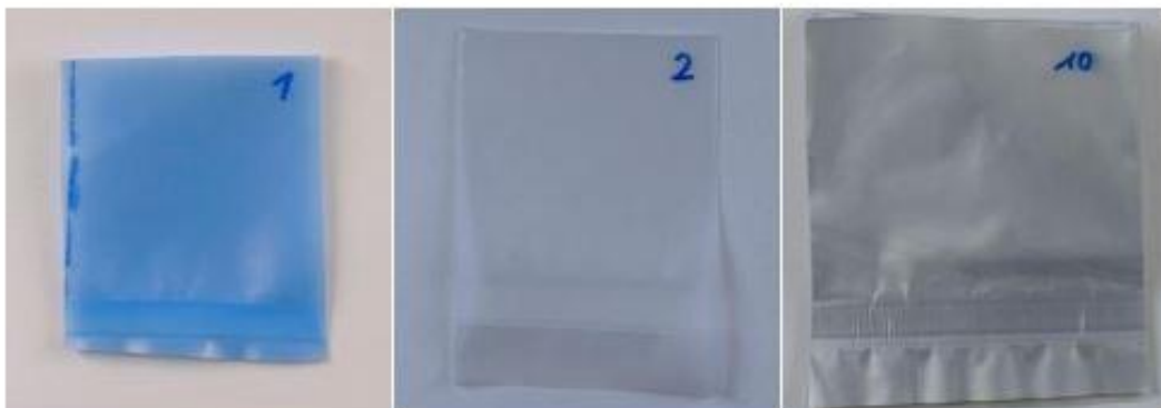
Fig. 2: Multilayer-film samples for transmission measurement
