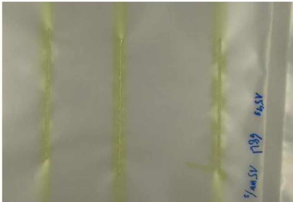
Fig. 7: Welding results at 15 mm/s feed rate visual transparent samples
