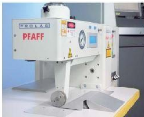
Fig. 9: Prototype of a sewing machine with integrated laser for welding of fabrics
