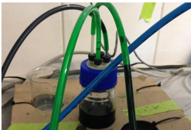
Figure 20. Final version of anolyte storage tank with insulated lid and extra nitrogen inlet.
