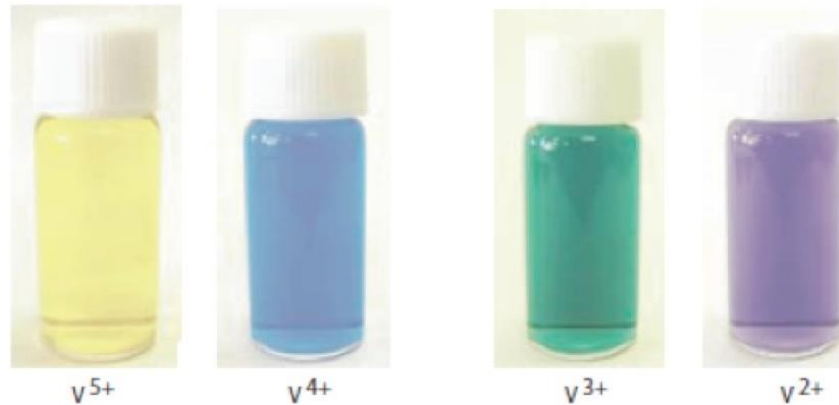
Figure 15. Visual appearance of diluted vanadium electrolyte at corresponding charge. (Ya-Ching Tseng, 2011)
