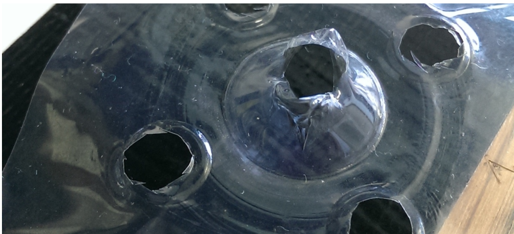
Figure 15. Bursting ETFE film.
