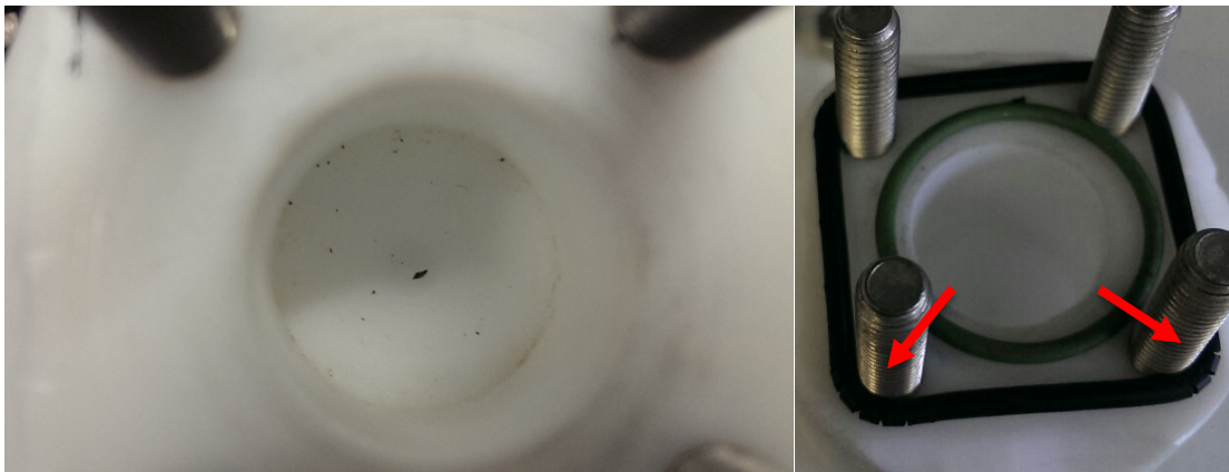
Figure 14. Brownish remains of a failed evaporated chamber, plastic has been removed (to the left) and cracking seals to the right.
