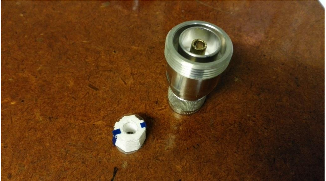
Figure 5. On the right side is the 7-16 male connector. On the left side is the sandwich assembly - the foam in the middle and CNT-covered disks on bottom and top.
