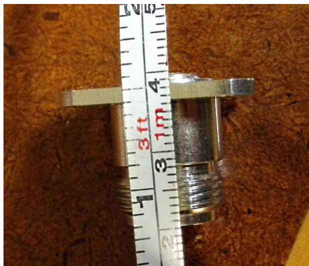
Figure 9. The length of the grinded type N panel mount adapter.
