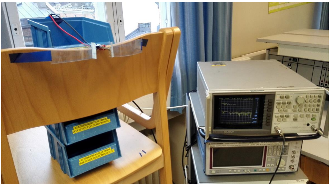
Figure 3. The CNT-covered film dipole antenna connected to the network analyser.
