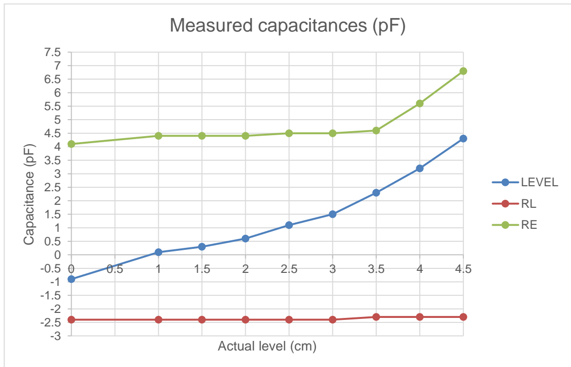
Figure 38. Capacitance measurement results with the Nucleo-STM32.
