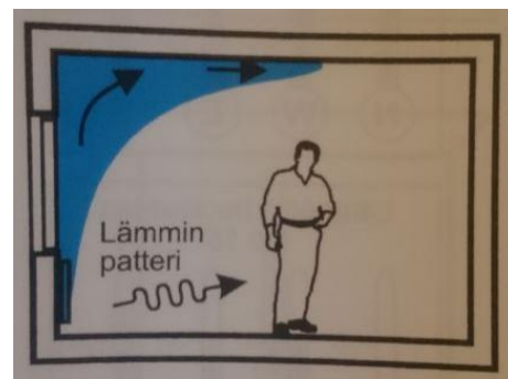
Figure 16. Heaters effect in front of a window
