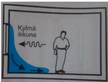
Figure 15. Cold windows effect on the air and causing draft
