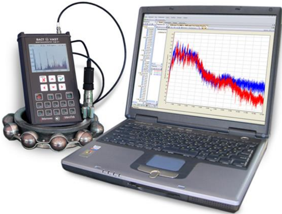
FIGURE 3. Russian portable vibration meter “SD-21” with original software. (VAST, 2016)
