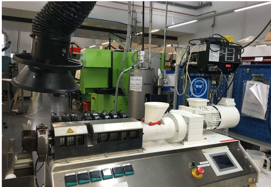
Figure 9: Extruder (Author, Arcada Plastic Laboratory 2016)
