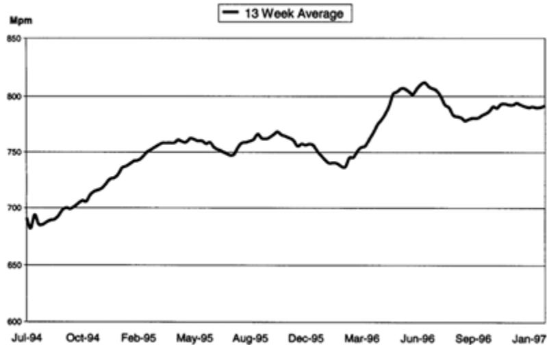
Figure 22. Speed was able to be increased from 750 meters per minute to 800 meters per minute (15)
