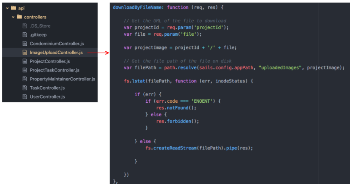
PICTURE 43: Picture showing list of controllers and method to get project image from the server
