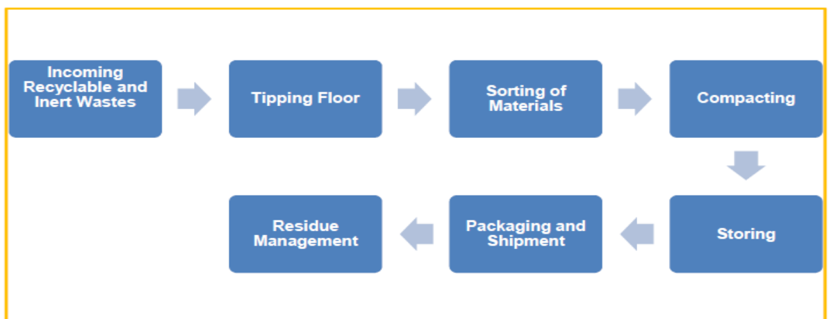
Figure 12. Flow chart showing Process of Material Recovery at MRF
