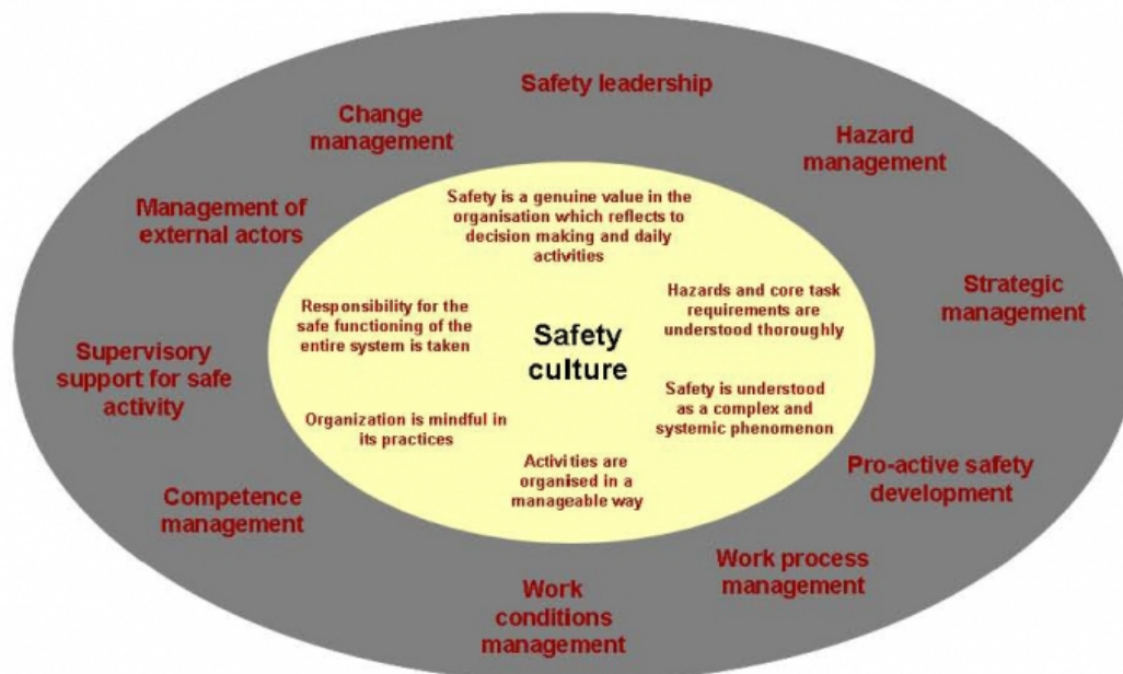
FIGURE 5. The model summarizes the criteria for good safety culture (in the inner circle) and the organizational functions that support the development of a good safety culture (outer circle) (Reiman & Oedewald 2009, 49).
