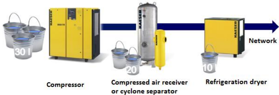
Picture 6. Condensate removal and drying (Kaeser 2014b)
