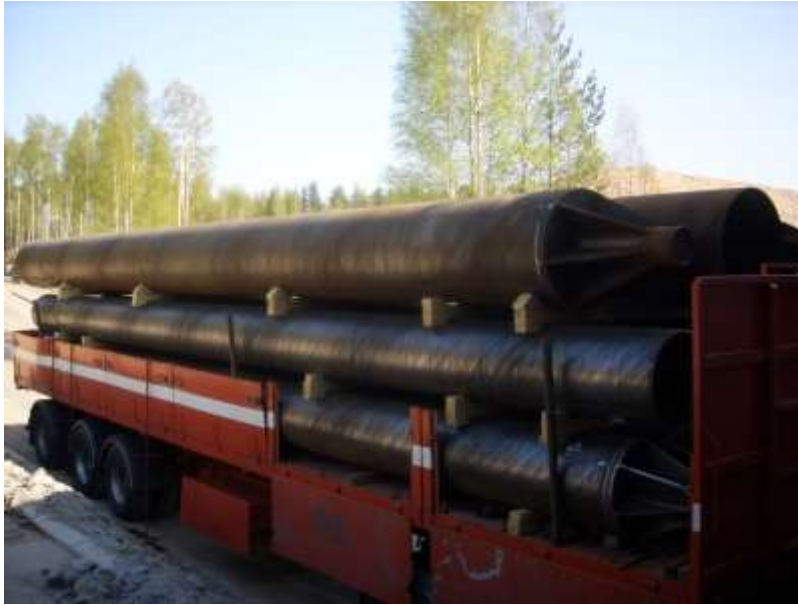
Figure 7. Steel pipe piles. (Teemu Kallio, 2006)
