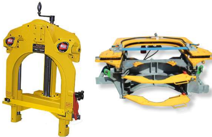
Figure 27. Guillotine pipe saw and SGS. (Guillotine Pipe Saw, 2009-2017; DTS Tooling, 2013)
