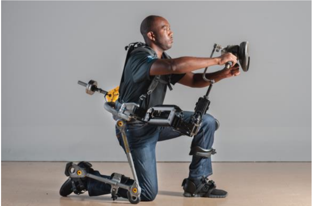
Picture 7. FORTIS personal exoskeleton for heavy tool use by Lockheed Martin (Lockheed Martin 2016)
