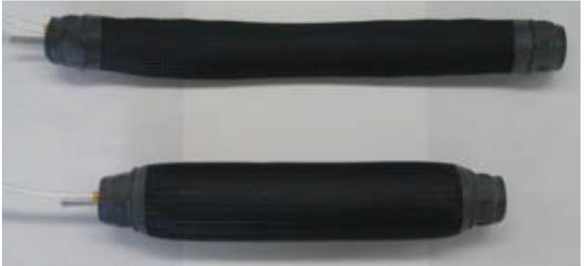
Picture 10. PAM to be used in the project, above in a pressurized state and below in an unpressurized state. (Kanda 2015)
