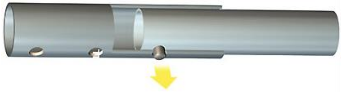
Figure 4. Internal telescopic tube locking device which was planned to be for adjusting the length of the frames. (Pete 2013)
