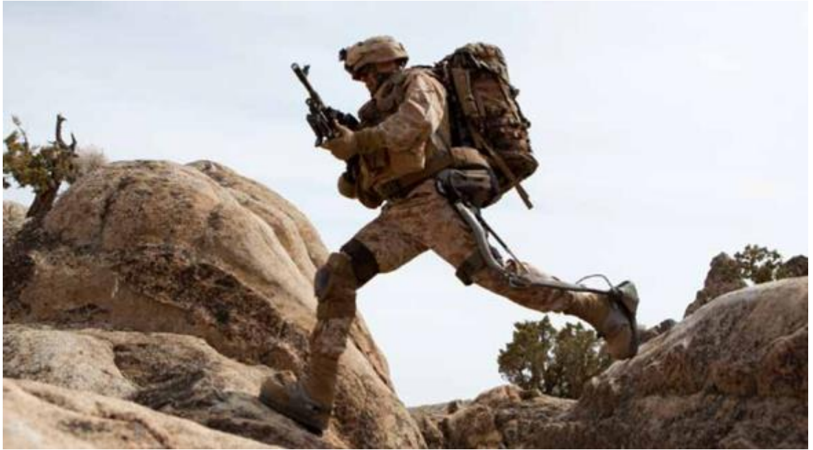
Picture 6. Human Universal Load Carrier - HULC by Lockheed Martin (Lockheed Martin 2012)
