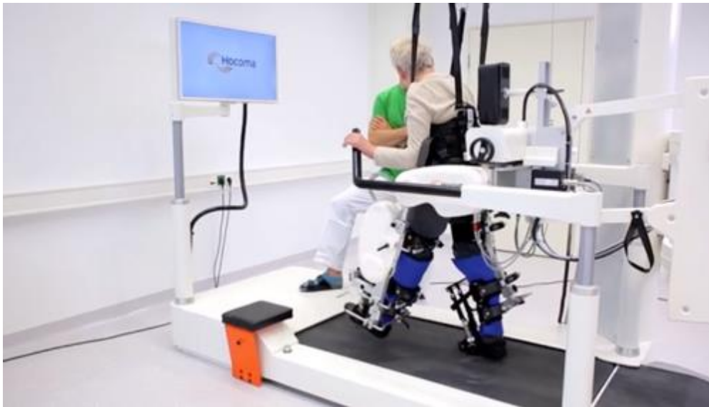
Picture 3. LokomatPro stationary LEE by Hocoma (Hocoma 2016)
