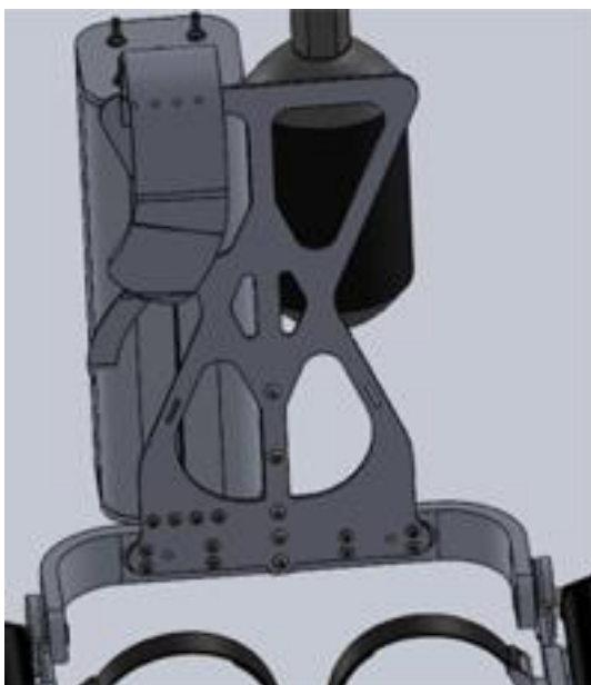
Figure 16. The actuator case and the tank connected to the system with 3mm sheet aluminum.
