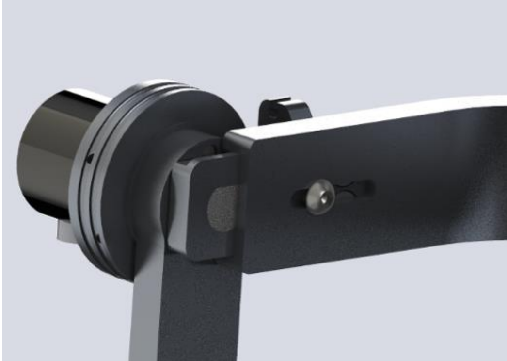
Figure 23. Shaped axle head and perfectly fitting machined slot for preventing twirling and making it possible to get reliable readings from angle encoder and sinking it to frame allows adjustment of the hip.
