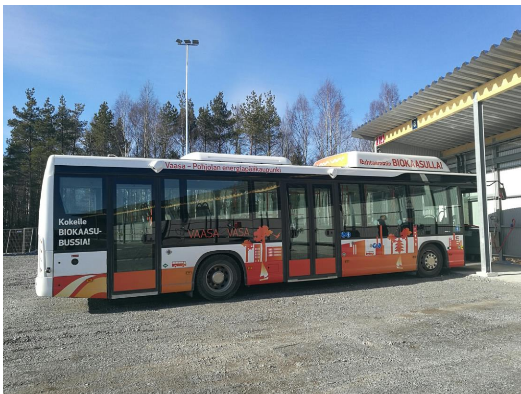
Figure 1. CNG bus in city of Vaasa at the slow filling station. Photo by the author.
