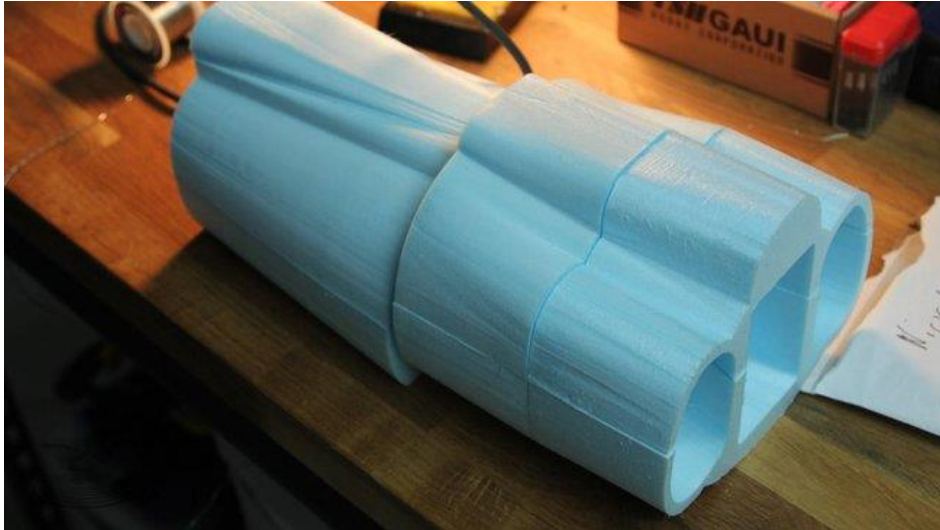
Figure 4 FliteTest. Hot-wire cut layers (3)
