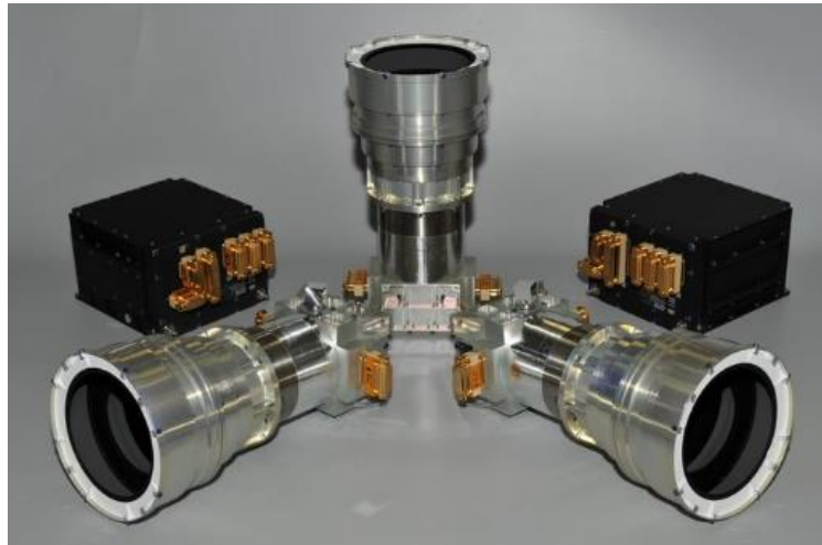
Picture 9. Hydra star-tracker currently flying on the ESA's Sentinel 3A satellite (ESA).
