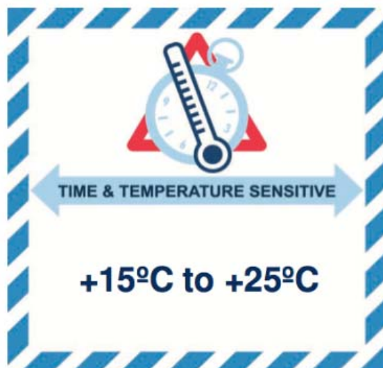
Kuvio 8. – IATA Time and Temperature Sensitive-tarra. (CoolChain Association 2012.)
