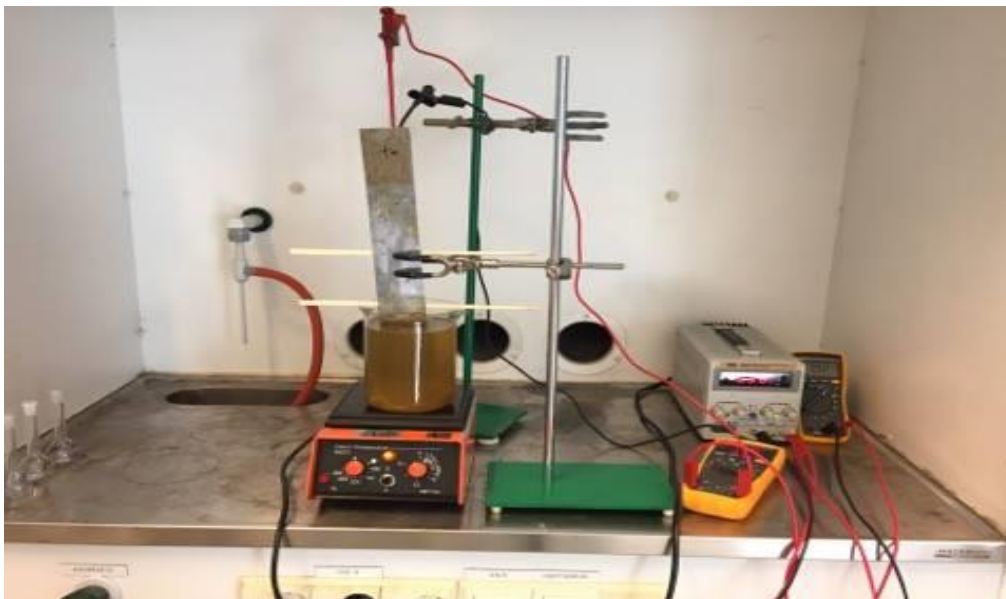
Figure 3 Experimental setup of electrocoagulation in the thesis
