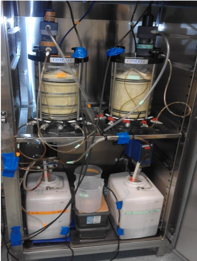
Fig 2. Experimental set-up for peat suspension test with propellers. Peat suspension was pumped from the canister through the soil column into the flow through cell where in situ pH, temperature-corrected conductivity and redox potential are measured every 15 minutes. Permeate from each experiment is collected in their respective measuring cylinders where the ex situ pH and temperature- corrected conductivity will be measured. The samples are collected and stored for further analyses.
