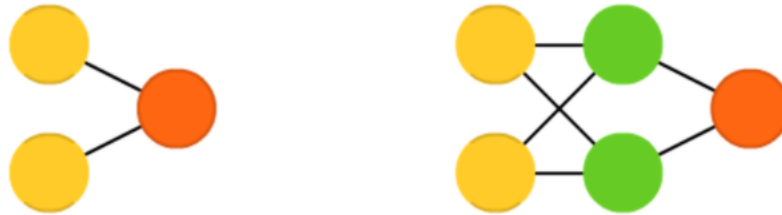
Figure 3. Fully connected (dense) NN structure. The left picture shows the least possible network.
