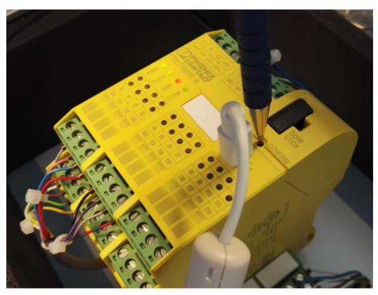
Figure **28.** CONFIRM – button is located in a hole right above Mini USB port. The button can be used with a pen or a match. A small click is enough for confirming the new program downloaded on the safety PLC.
