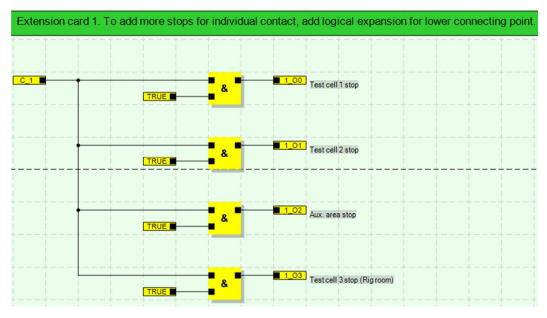
Figure **30.** Common panel CJU901 extension card program, each extension card program has its own program network.
