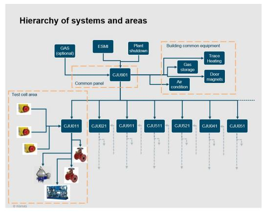
effective inside the emergency stop area, unless necessary for safety of the area. The basic principle of the hierarchy can be seen in Figure 4.
