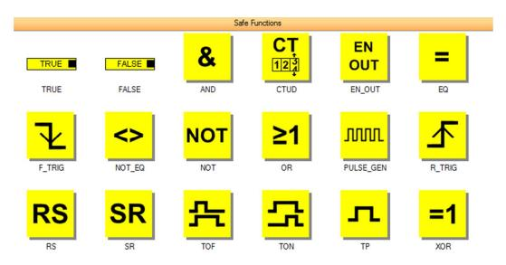
Figure 24. Safety functions available for FBD programming of safety PLC.
