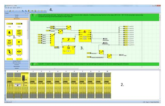
Figure 23. The SAFECONF – main window. 1. Tool Box, drag & drop logical functions for toolbox. 2. Hardwire Editor, modify hardwire suitable on project and program. Add hardware for toolbox menu with drag & drop. 3. Program Network, add and connect logical functions, inputs and outputs for program network. 4. Menu for properties and tools.
