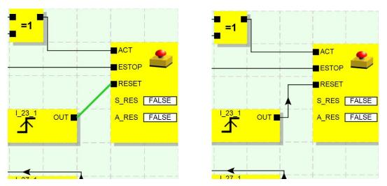
Figure **26** (left). If connection is allowed the straight line appears in green colour. If connection is not allowed line is red and connection is not made. Figure **27** (right). Successfull connection.
