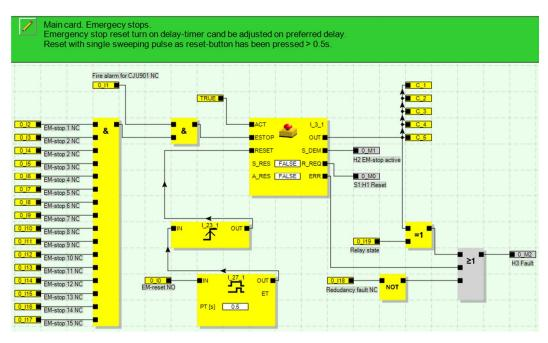
Figure **31.** CJU541 area main network. Similarities between common panel and test rig area emergency stop is notable.
