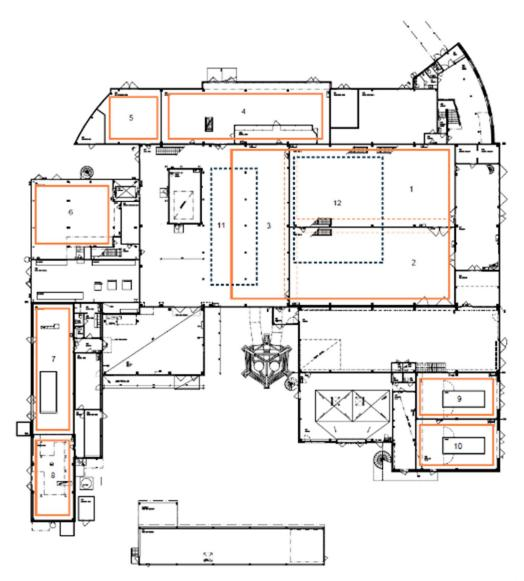
Figure **2.** Existing emergency stop areas in the building. Orange lines shows the  $1^{\text{st}}$ . floor emergency stop areas and blue dotted line the  $2^{\text{nd}}$ . floor emergency stop areas.
