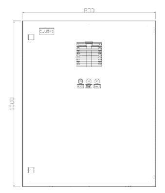
Figure **19.** Face layout for emergency stop cabin CJU541. The electrical cabin doors of the emergency stop system are mostly identical.
