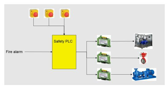
Figure 5. Technical principle of the emergency stop area.
