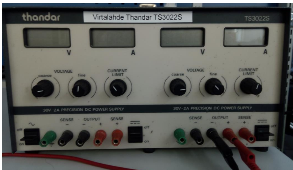
PICTURE 20. External power supply "Virtalähde Thandar TS3022S" (Photo: Jordy Declercq 2017)
