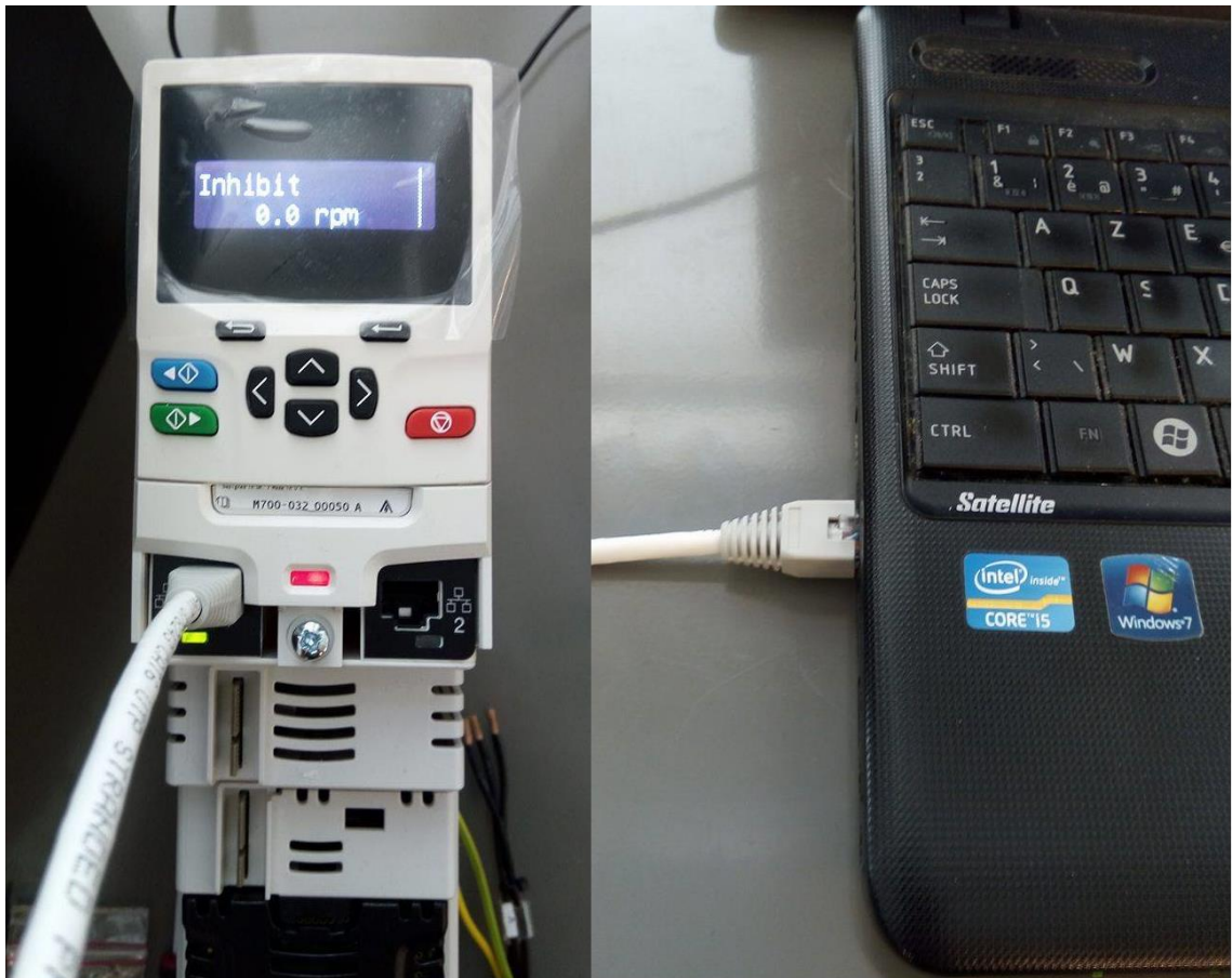
PICTURE 21. Ethernet connection between the Unidrive M700 and a computer (Photo: Jordy Declercq 2017)
