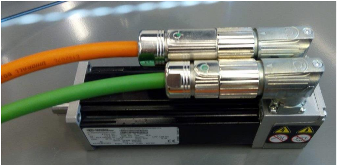
PICTURE 15. Connection of power supply and encoder cable to servo motor (Photo: Jordy Declercq 2017)
