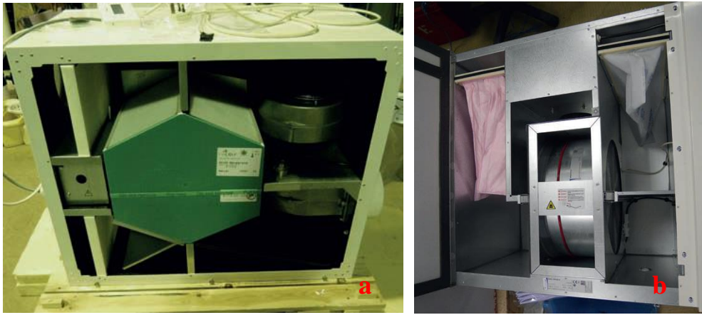
FIGURE 17. A counter-flow plate heat exchanger (a). A rotating heat exchanger (b).
