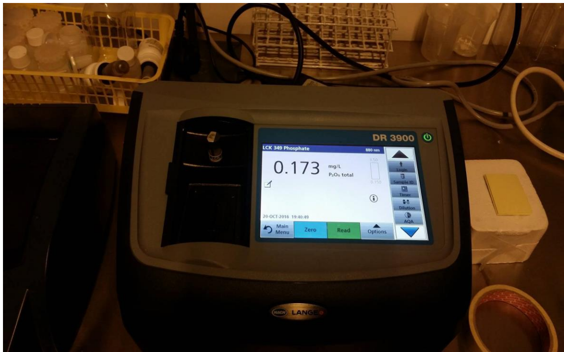
Figure 16. Nitrogen and phosphorus test using Hach/Lange Spectrophotometer DR 3900
