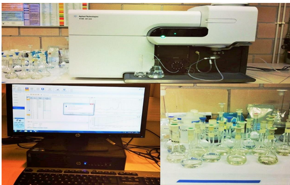
Figure 15. Iron test using 4100 MP-AES technology
