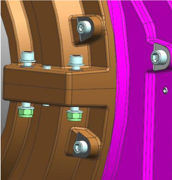
Figure 11. Horizontal bolts used as fastening point
