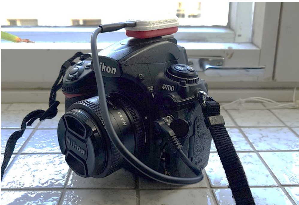
Figure 20: The finalized product, seated in the hot shoe on a camera. The cable goes from the product to the camera remote socket
