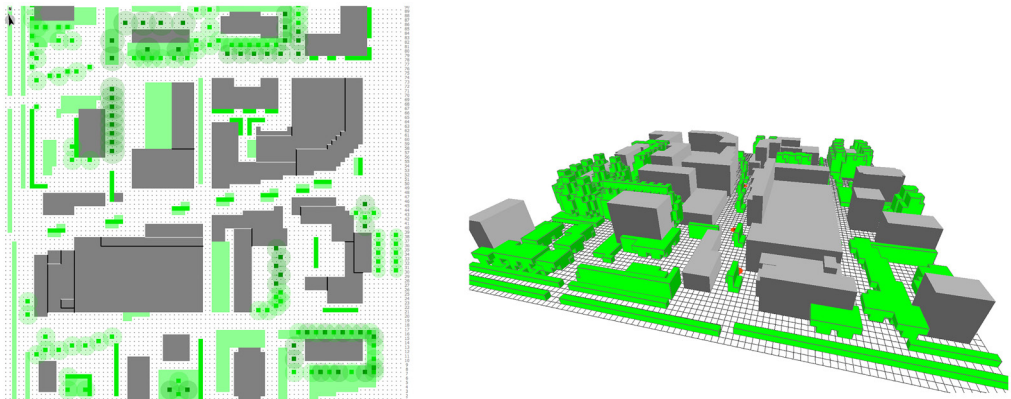
Figure 2: 2-dimensional bird-view (left) and 3-dimensional (right) ENVI-met view of the Tikkuraitti pedestrian area (plants and buildings). (Figure: ENVI-met software adapted by Achim Drebs).
