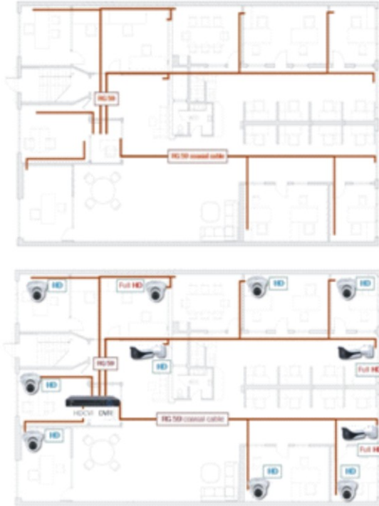
Picture 2. The previously installed and used coaxial cable installation (on the top), which works as the basis for installing HD and Full HD 1080p HD CVI camera system (in the bottom) 425
