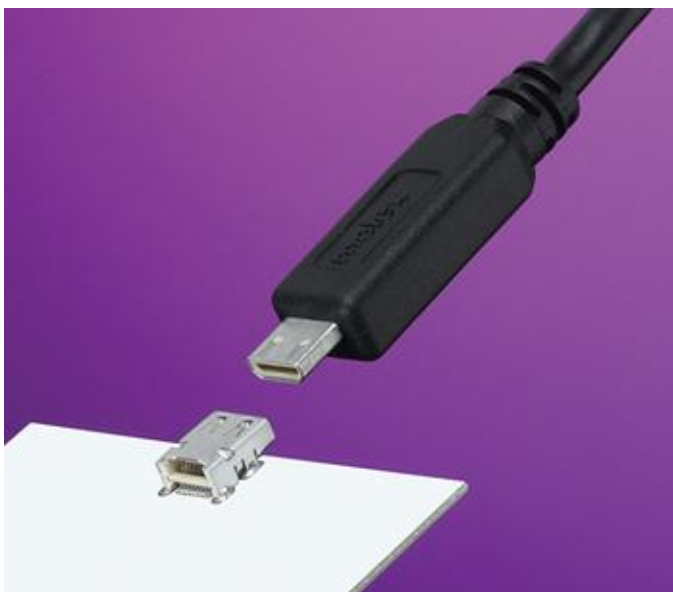
Figur 3. HDMI Typ D kontakt (EE Times Group, a Division of United Business Media LLC. 2010 )
