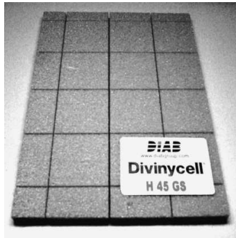
Figure 3: Divinycell H45GS foam core before lamination
