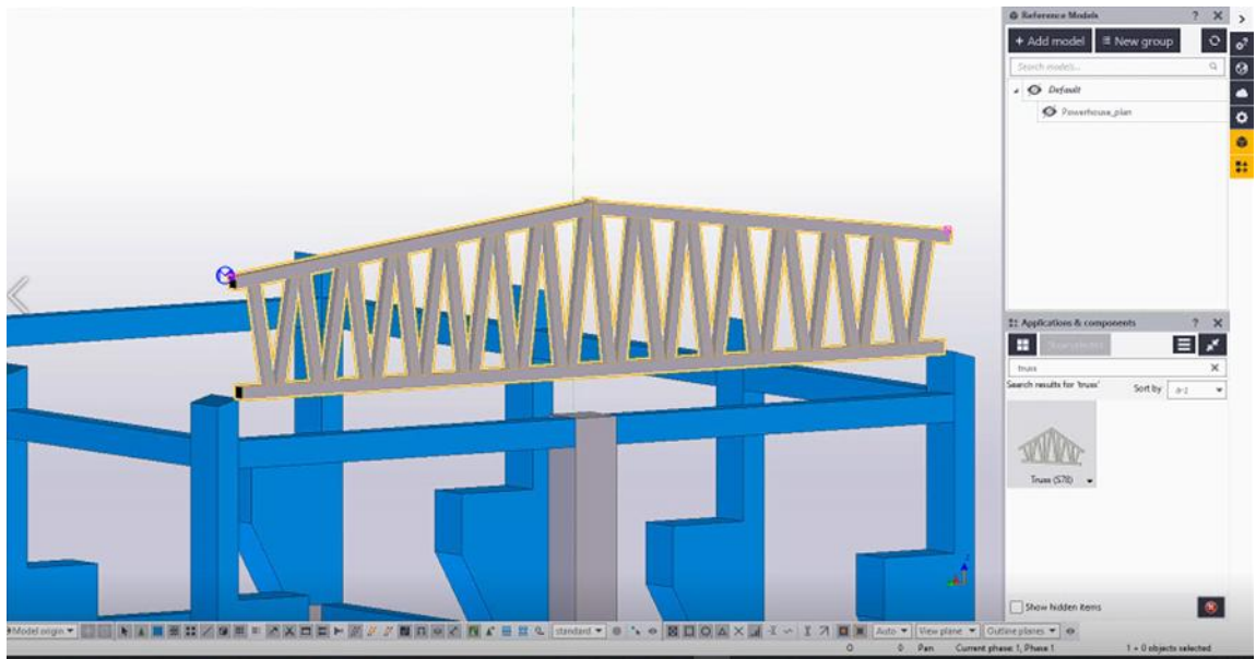
Figure 13. Adding truss on top of columns for the roof
