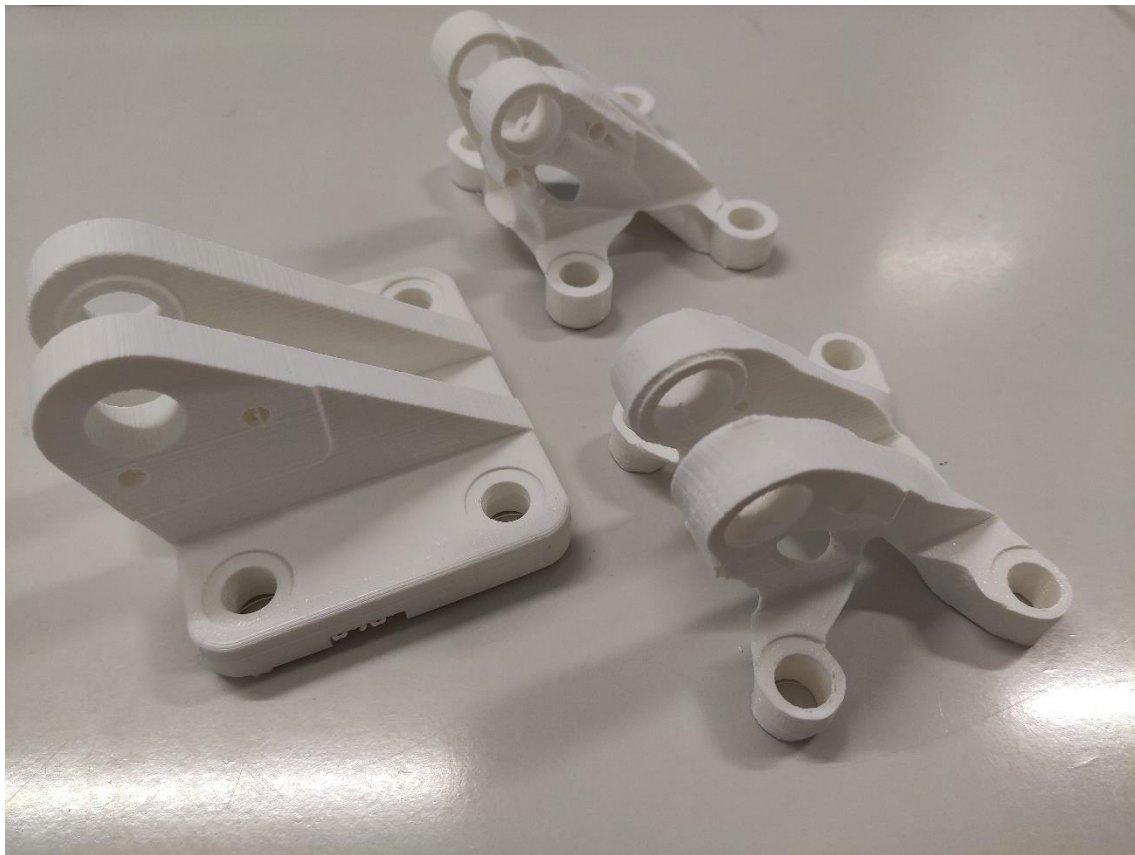
Figure 26. 3D Printed mounting brackets with Parker standard part to the left, solid Thinking Inspire on the top and SolidWorks optimized to the right (Oliver Folger, 2019)
