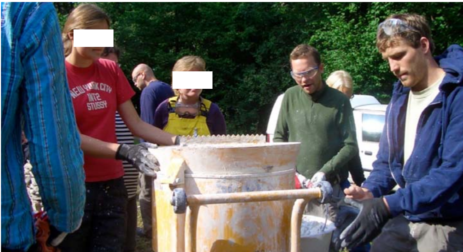
Figure 12. Making bigger quantities of lime render by using a roller pan mortar mill.
