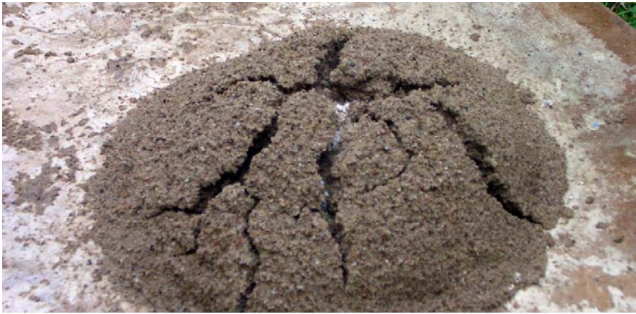
Figure 9. The burned lime is reacting with the added moisture. It expands to double its volume and releases heat.
