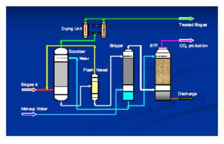
Figure14. Scheme of biogas treatment system
