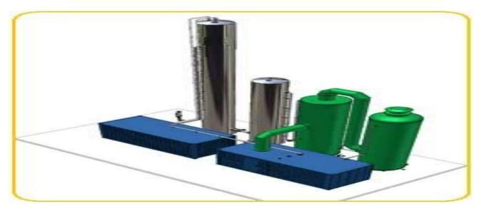
Figure 13. 3D model of biogas treatment unit 250 m3/h capacity [20]
