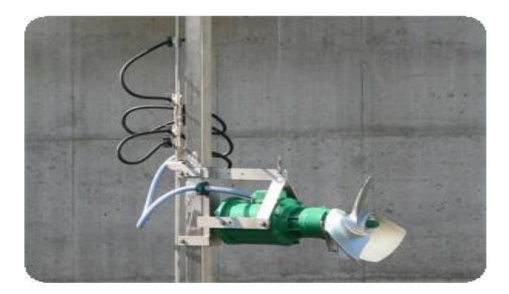
Figure7. Submercible agitator [14]
