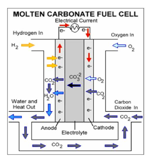
Figure 22. Molten Carbonate Fuel Cells [9]
