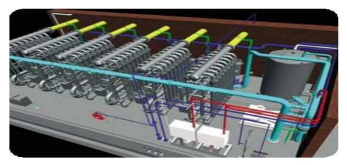
Figure 20. 3D model of membrane treatment unit [23]
