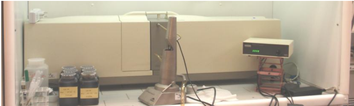
Figure 5. Malvern Mastersizer device[6]
