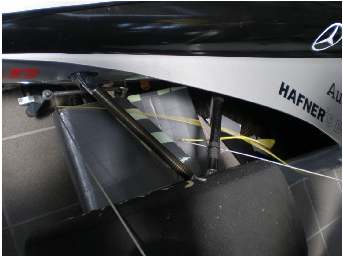
Figure 20 The air flow over the suspension modifications
