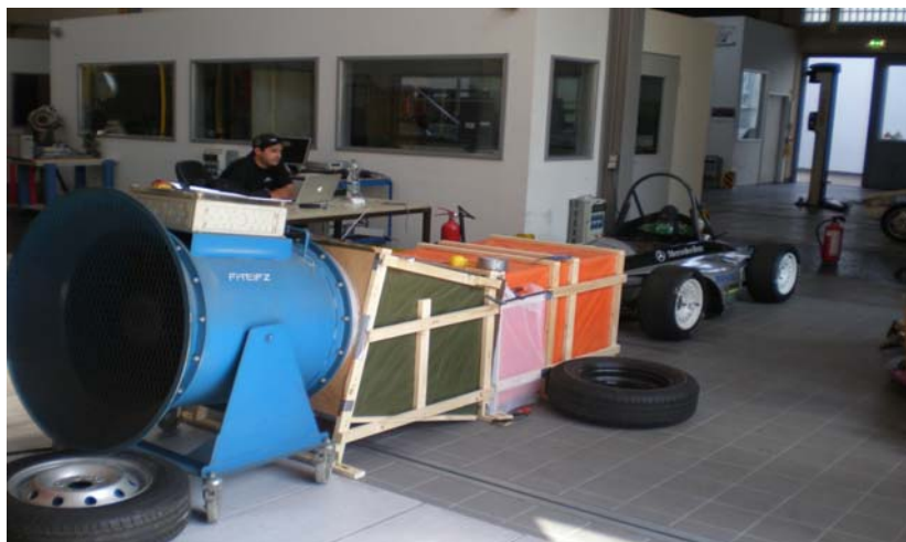
Figure 2 The flow straightener and the test bench
