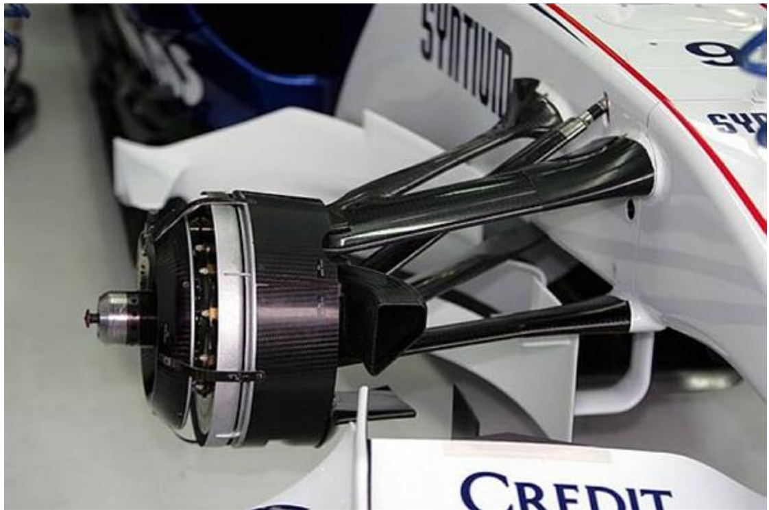
Figure 12 Formula 1 suspension elements /11/
