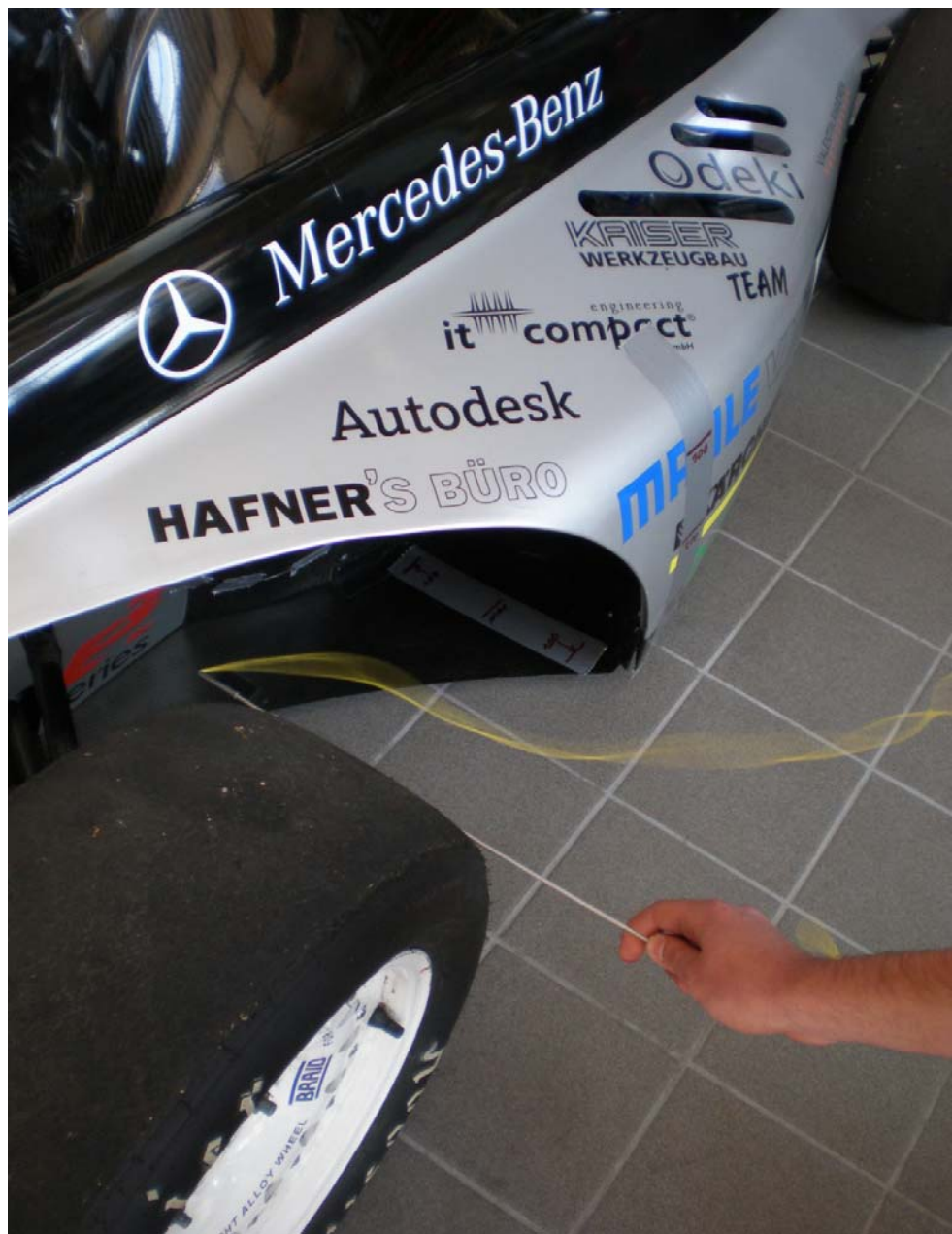
Figure 13 The original duct during baseline test
