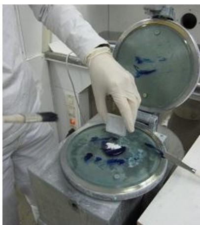
Figure 72: Application of the ink and filler on the muller (Kulmala 2010a: 1).
