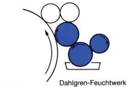
Figure 6: Conventional dampening system (Viluksela 2005: 17).
