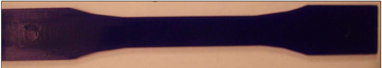
Figure 17 Shape of a dog bone made out of SABIC PP 505P (Arcada plastic laboratory, 2012)
