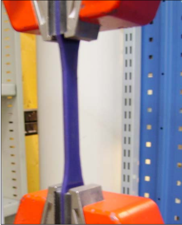
Figure 18 A dog bone being tested with the testometric tensile testing machine (Arcada plastic laboratory, 2012)
