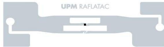
Figure 1.3 A type of UPM Raflatacs UHF Gen 2 chip displayed in natural size format. The black dot is the microchip and the hammer-like structure around it the antenna. Antenna measurements 76.5 x 23 mm.
