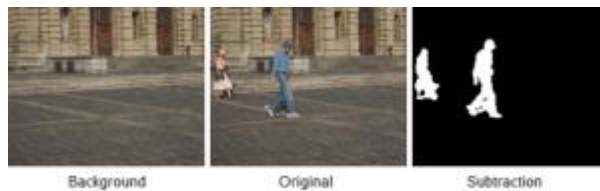
Picture 22. Machine Vision Based approach (Background segmentation for extracting the silhouette picture)
