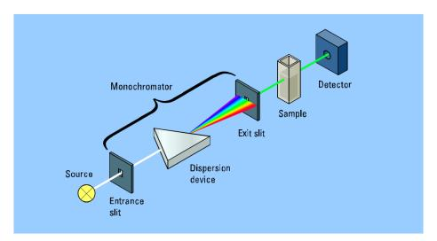
GRAPH 1. The principle of work of UV-Vis spectrophotometer (adapted from Davison college 2012)
