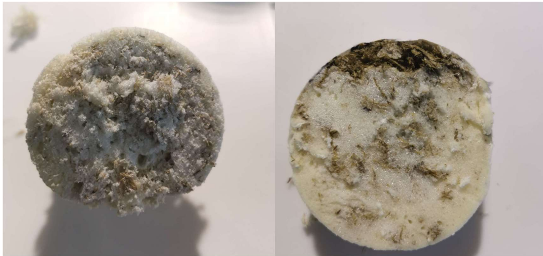
Figure 22: Typha latifolia -PU foam with open-cell structure (left). Typha latifolia -PU foam with closed-cell structure (right).
