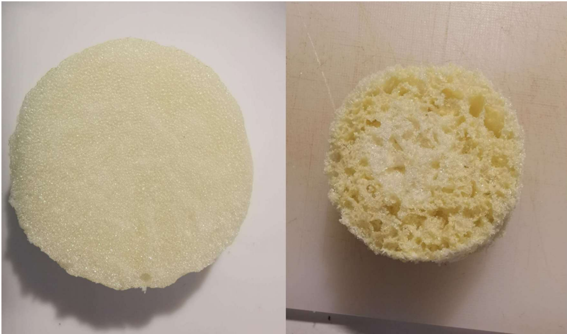
Figure 16: A closed-cell polyurethane foam with 50/50 ratio of resin and catalyser (left). An open-cell water blown rigid polyurethane foam with ratio of 5/16 of resin, 5/16 of water and 6/16 of catalyser (right).
