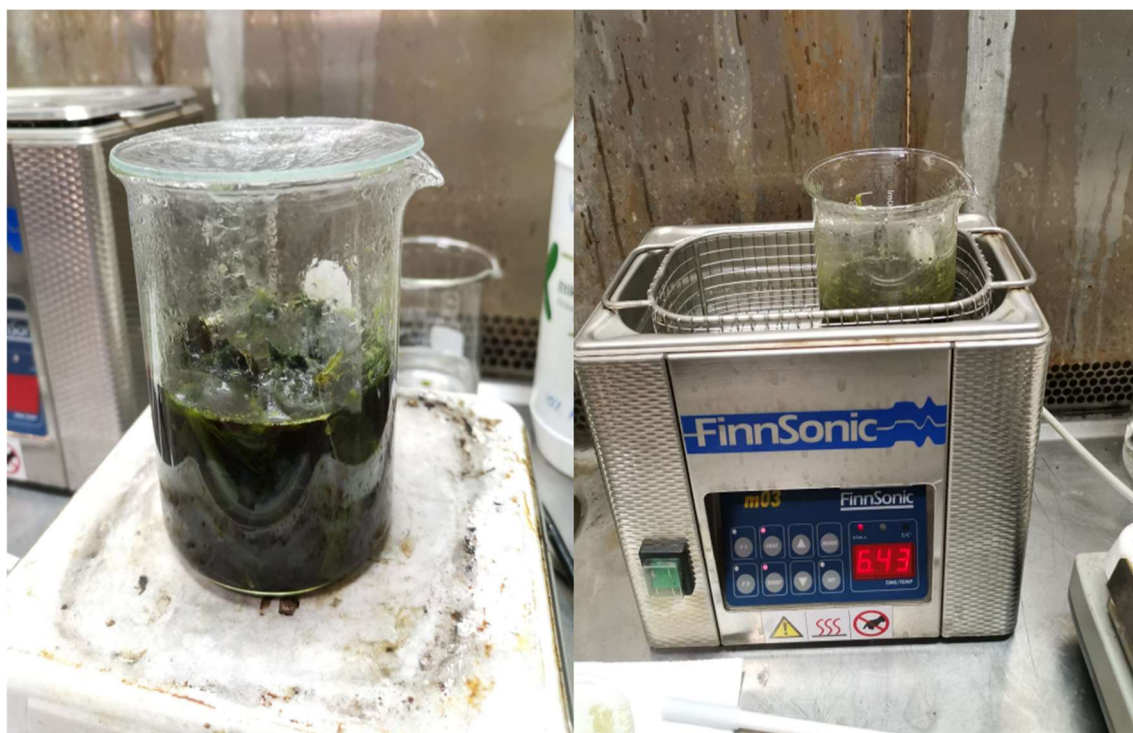
Figure 10: Left: Typha leaves in sodium hydroxide. Right: The solution in an ultrasonic bath.
