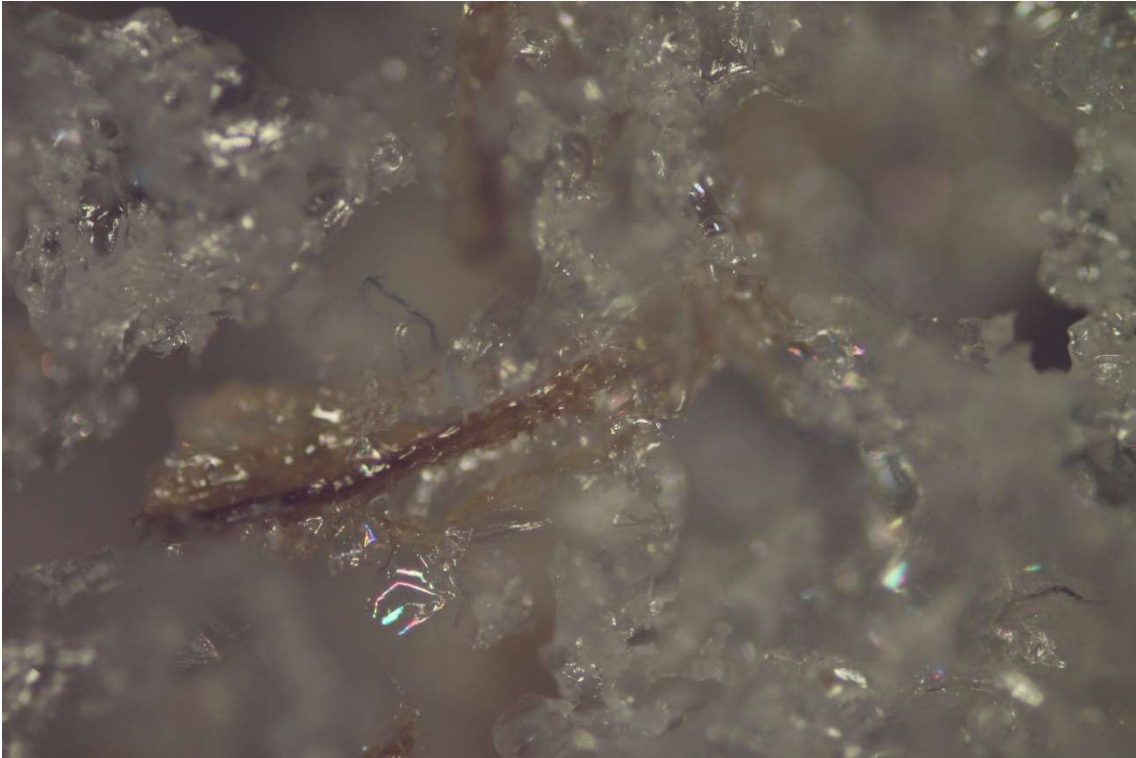
Figure 28: Typha latifolia-PU foam with open-cell structure, seen in Figure 22 at section 4.3, under a microscope.
