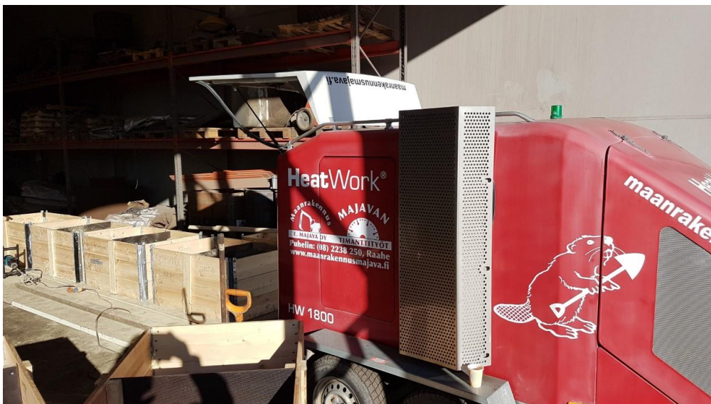
PICTURE 2. Heatwork HW1800 Thermal power station
