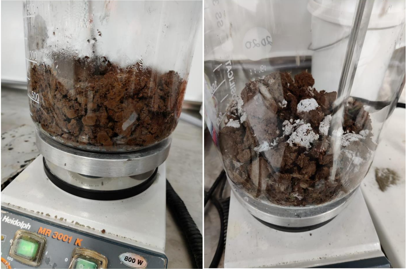
PICTURE 5. Zinc ferrite before and after an eight hour drying session at 70°C
