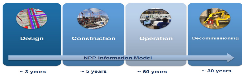
PICTURE 1. Typical nuclear power project life cycle (IAEA Nuclear Energy Series NR-T-1.18).
